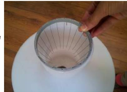
The upper part of the Separator (Cyclone) should rest upon the Wire-ring.
