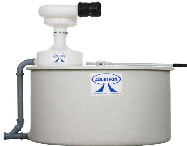
AQUATRON 4x200 system. All the 4x system are built to composte the faeces and papers in separate chambers within the composting unit. Once composted the volume is reduced by 75-90%
